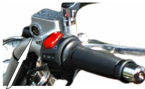
Front brake fluid level window. The fluid should not be below the window.
