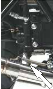
Adjusting push rod and lock nut.
